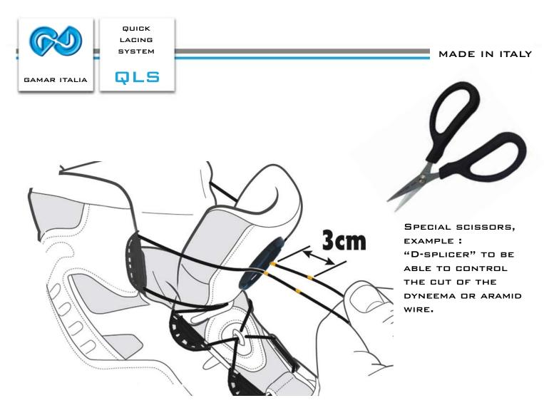
CUT THE WIRE IN THE RIGHT SIZE TO PERMIT THE COMPLETE OPENING OF THE SHOE PLUS 3CM AT EACH EDGE.
