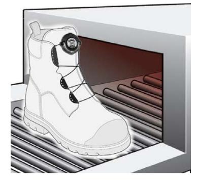
WE SUGGEST NOT TO EXCEED 70°C/80°C WHEN THE SHOE GOES INSIDE THE STABILIZATION OVEN.
